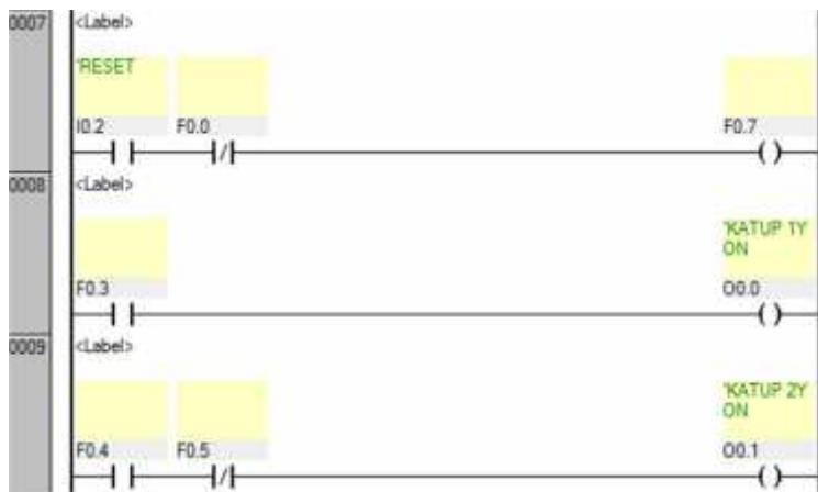
*Gambar 4.50 Ladder Diagram percobaan 19*
