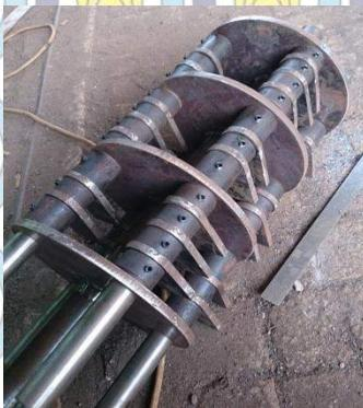
Gambar 4.8 : Assembly hammer
