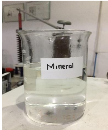
Gambar 3.3 Minyak Mineral (Shell Diala B)
