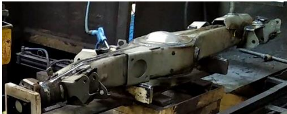
Gambar 2.2 Housing dari differential gear
