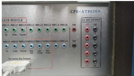
Gambar 4.1. Output DC panel kontrol
