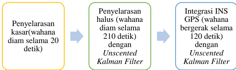
Gambar 3. 1 Diagram alur sistem INS-GPS
