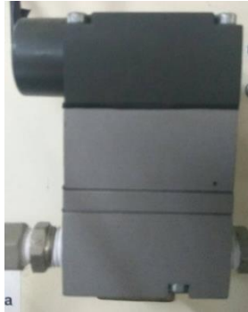
Gambar 2. 12 I/P Converter pressure process Rig 38-714
