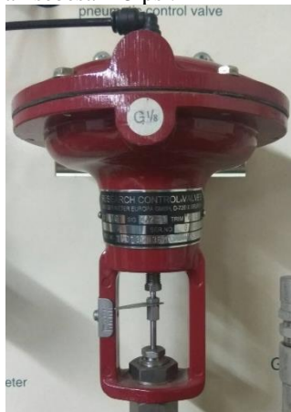
Gambar 2. 5 Pneumatic control valve pressure process Rig 38-714
