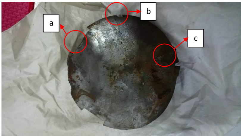
Gambar 3. 3 Daerah Pengambilan Spesimen (a) Initial Crack (b) Propagation (c) Final Crack
