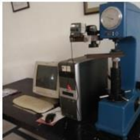
Gambar 3. 6 Alat Uji kekerasan Universal Hardness Tester HBRV 187.5A (Teknik Material, 2018)
