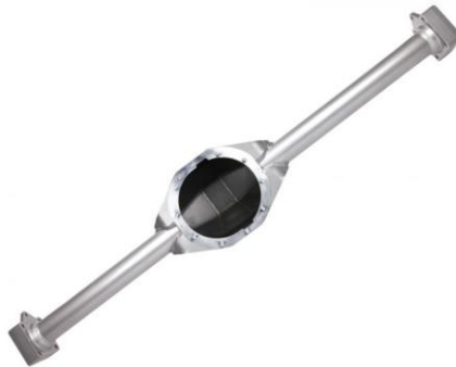
Gambar 2. 6 Housing of Differential Gear
