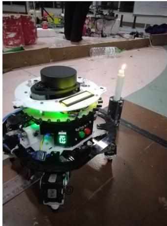
**Gambar 4.4** Pengujian sensor *Phototransistor*.
