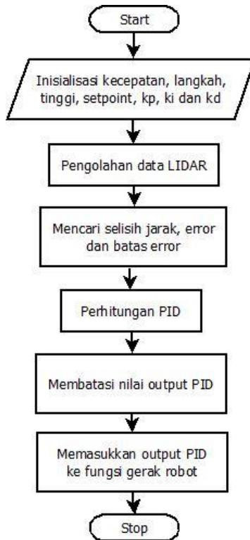
**Gambar 3.21** Flowchart perancangan PID.
