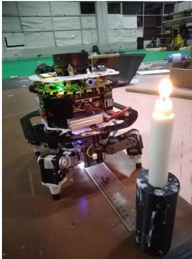
**Gambar 4.3** Pengujian sensor UVTRON.
