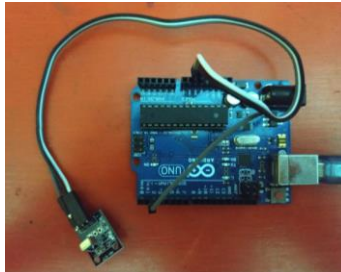
Gambar 4.2. Setting pengambilan data remote AC
