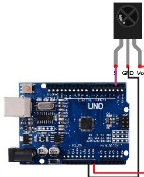
Gambar 3.17. Wiring of decoder AC Remote
