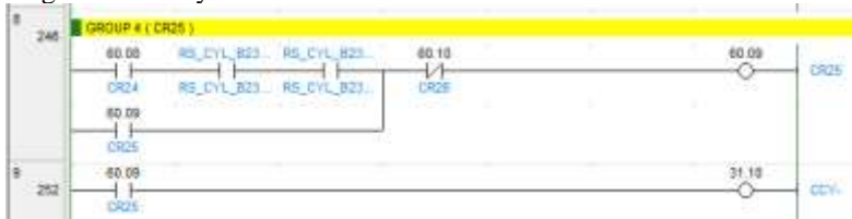
Gambar 3. 28 Ladder Diagram CR25
