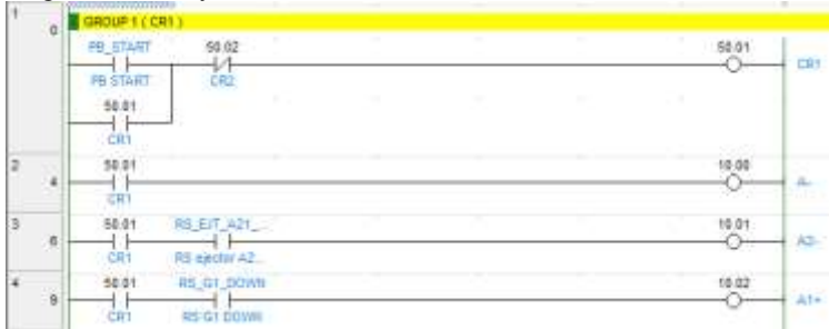
Gambar 3. 4 Ladder Diagram CR1
