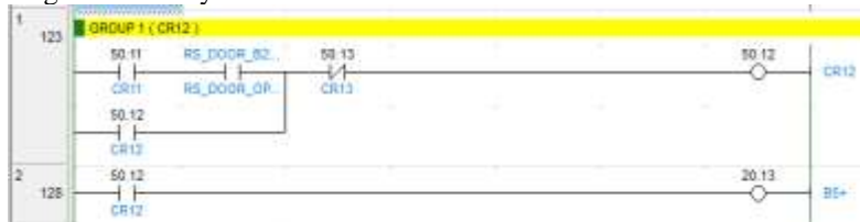
Gambar 3. 15 Ladder Diagram CR12
