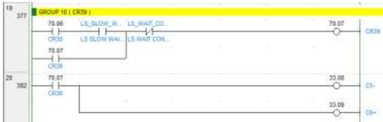
Gambar 3. 42 Ladder Diagram CR39
