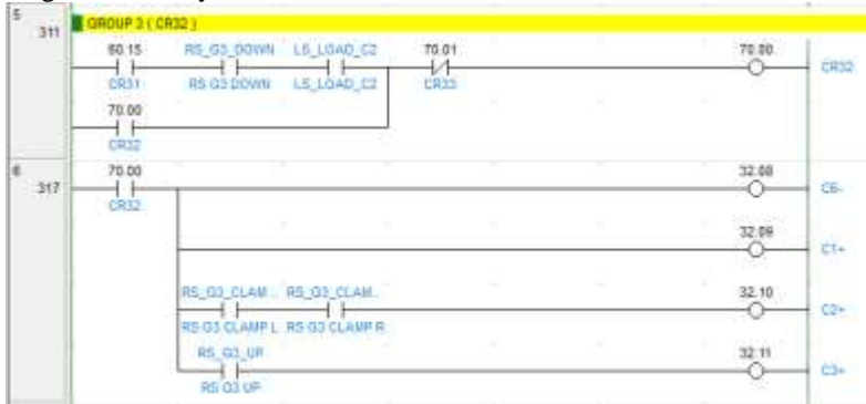
Gambar 3. 35 Ladder Diagram CR32
