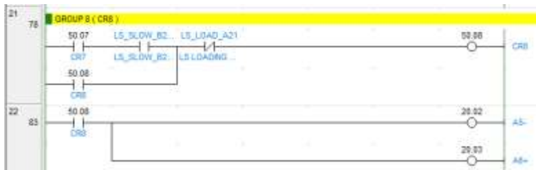
Gambar 3. 11 Ladder Diagram CR8
