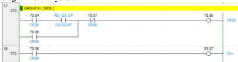
Gambar 3. 41 Ladder Diagram CR38
