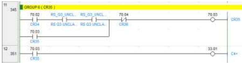
Gambar 3. 38 Ladder Diagram CR35
