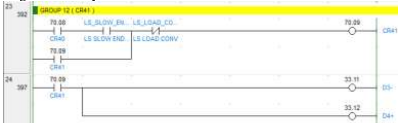
Gambar 3. 44 Ladder Diagram CR41
