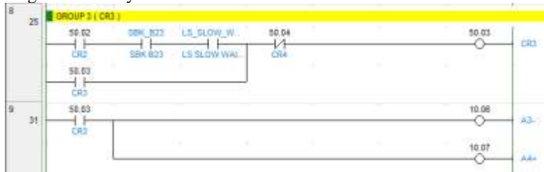
Gambar 3. 6 Ladder Diagram CR3
