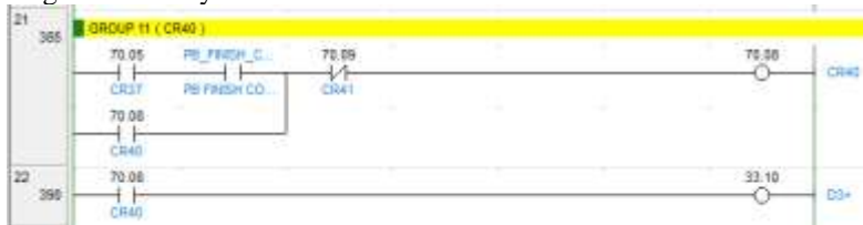
Gambar 3. 43 Ladder Diagram CR40
