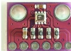
**Gambar 2.14** Modul sensor tekanan barometrik BMP280
