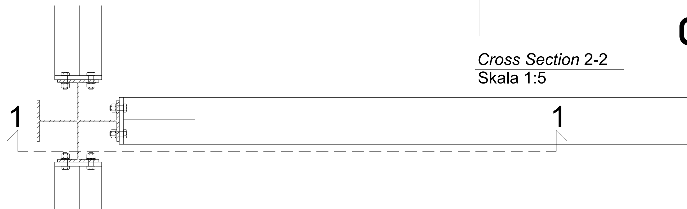
Perkuatan Balok WF396, L=9m Join B'-A' dan E-F, As 1' Skala 1:5
