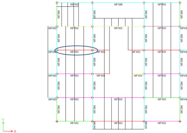
Gambar 5. 3 Lokasi WF450, L=9m
