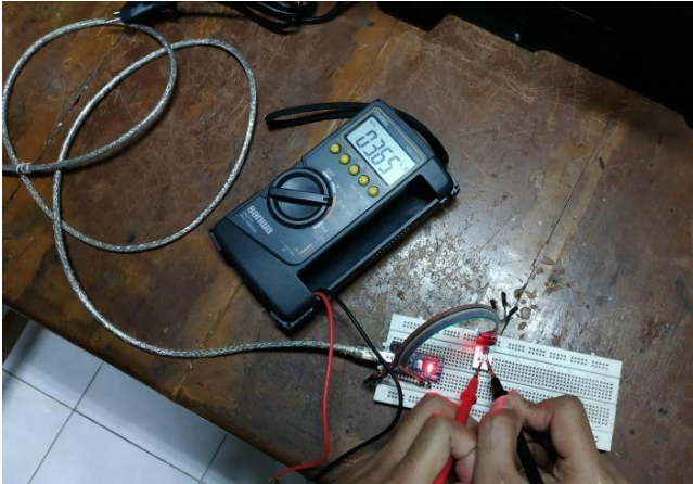
Gambar 4.3 Proses pengujian digital potentiometer X9C103.
