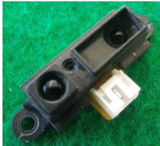
**Gambar 3.21** Sensor Jarak Sharp GP2D12
