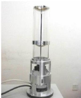
**Gambar 2.16** Kamera *Omnidirectional* [22]
