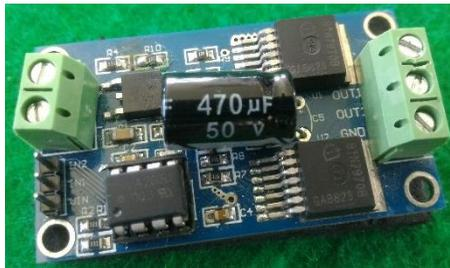
**Gambar 3.30** Modul Driver Motor BTN7970
