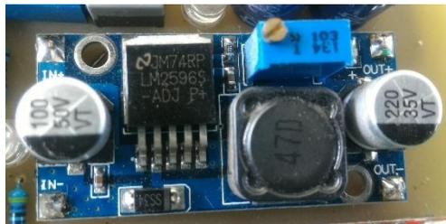
**Gambar 3.16** LM2596 *Buck Converter*
