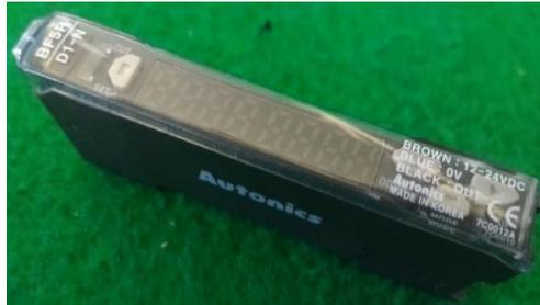
**Gambar 3.22** Sensor Garis Autonic BF5R
