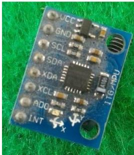
**Gambar 3.24** Sensor IMU MPU6050
