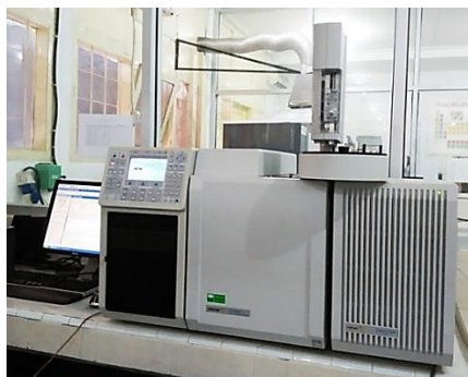
Gambar 2.12 Instrumen GC-MS Varian Saturn CP-3800/22000MS (LTSIT, 2016)
