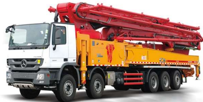
Gambar IV. 5: Concrete Pump Truck
