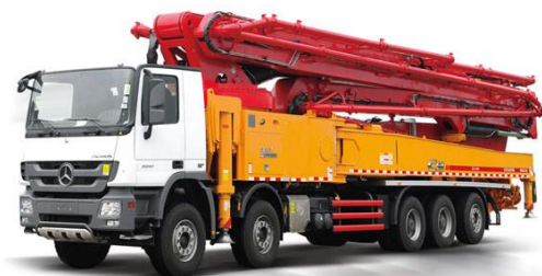
Gambar 2. 8 Concrete pump truck
