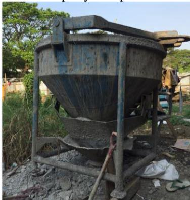
Gambar 2.11 *Concrete Bucket*
