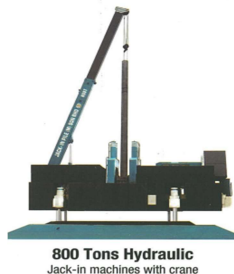
Gambar 16 Jack in Pile Sumber : Google.com
