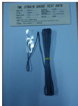
(a) Strain gauge FLA 2-11
