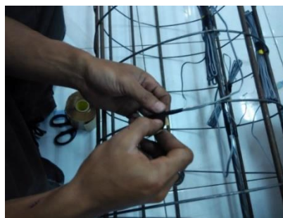
(a) Strain gauge tulangan PC bar (b) Strain gauge tulangan spiral
