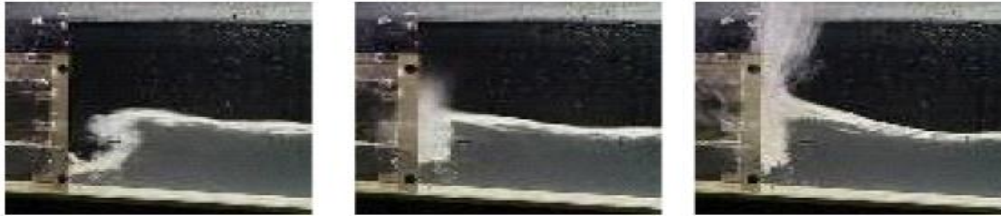
Gambar 2.10 Kondisi overtopping impulsive (Kim, 2010)
