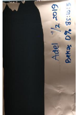
Hasil coating lembaran anoda A01P kering
