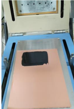
Hasil coating lembaran anoda basah
