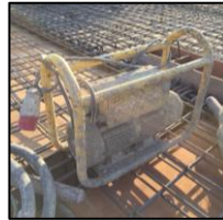
Gambar 2. 12. Concrete Vibrator Sumber : PT Jaya Kusuma Sarana
