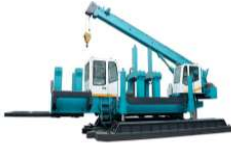
Gambar 2.13 Hydraulic Jack in Pile
