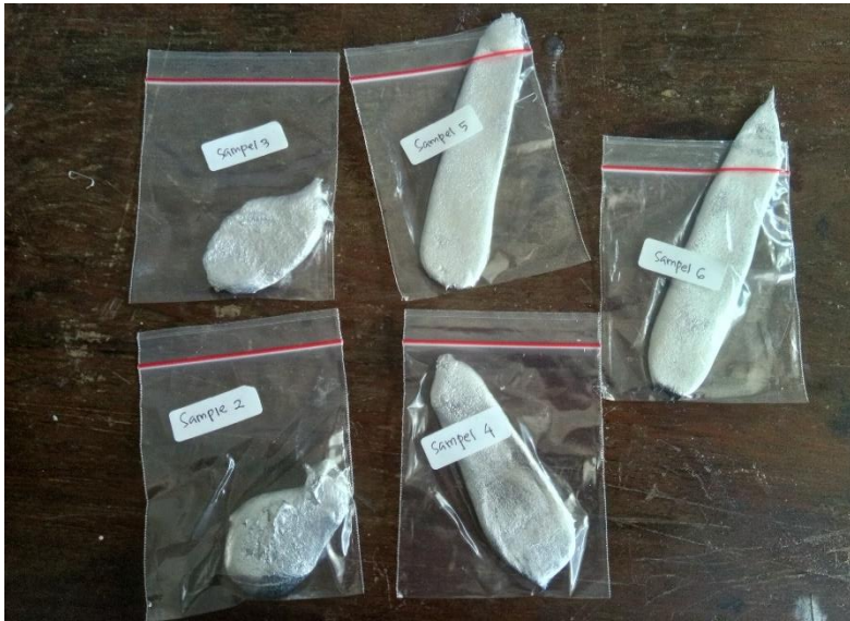
Gambar 3.2. Sampel paduan aluminium-silikon hasil coran
