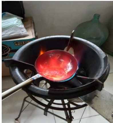
Gambar 3.1. Proses peleburan paduan aluminium
