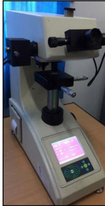
**Gambar 3.10** Alat Pengujian Kekerasan Microvickers Hardness
