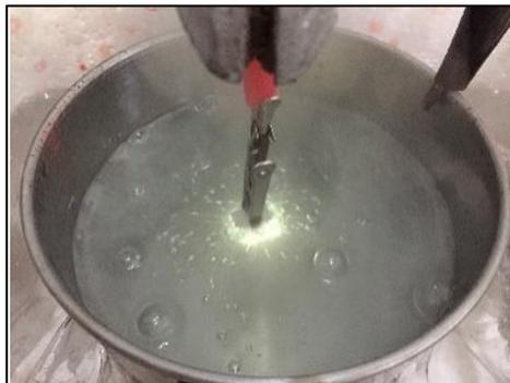
**Gambar 4.1** Proses PEO (*Plasma Electrolytic Oxidation*)
