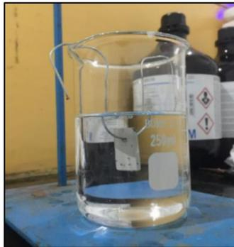
**Gambar 3.5** Proses *Dip Coating*
