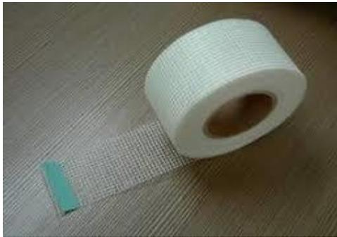
**Gambar 3. 2** *Mesh Tape Fiberglas*
