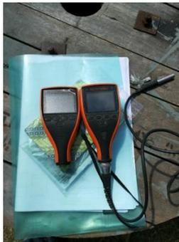
**Gambar 3.5** Alat Uji Ketebalan *DFT Electomer* (Elcometer, 2016)
