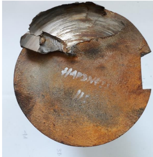
Gambar 3. 3 Penampang Patahan Circulating Water Pump Shaft (Dokumen Pribadi)
