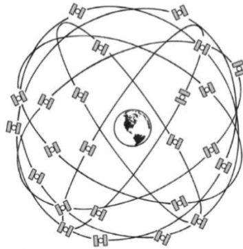
Gambar 2. 3 Global Positioning System (GPS), konfigurasi 24 satelit (Seeber 2003)
