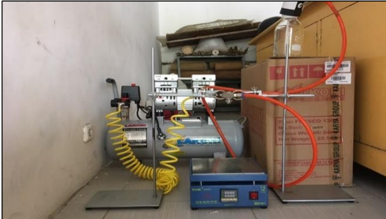
Gambar 3. 2 Rangkaian Alat Spray Pyrolysis Deposition
