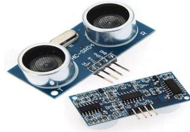
**Gambar 2. 1. Sensor Ultrasonik HC-SR04**
