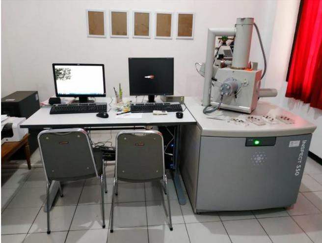
**Gambar 3.13** Alat SEM/EDX Dept. Teknik Material ITS
