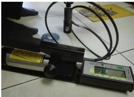
**Gambar 3.14** Alat *Pull Off Test*
