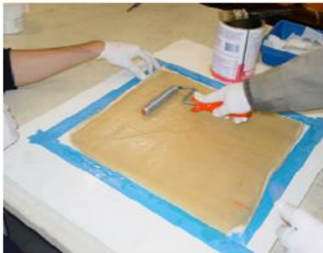
Gambar 2. 18 Hand Lay Up Proses (Yuvaraj, 2016)
