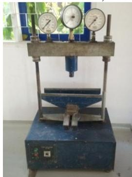
**Gambar 3. 14** Mesin Uji Bending
