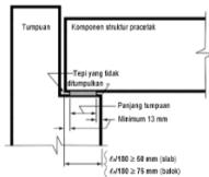
Gambar 3.11 Detailing Beton Pracetak (Sumber:RSNI 2847:2018)
