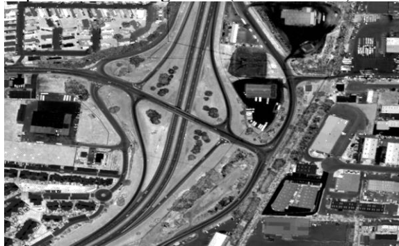
Gambar 2. 10 Hasil LiDAR Intensity Image (Munjy 2011)
