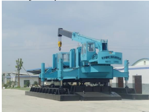
Gambar 2. 3 Hydraulic Jack In Pile 320 T
