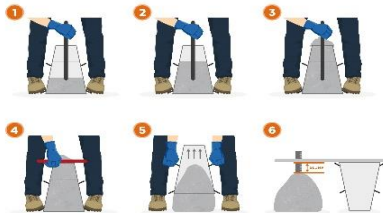
Gambar 4. 4 Test Slump
