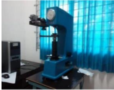
Gambar 3.6 Alat Uji kekerasan Universal Hardness Tester HBRV 187.5A (Teknik Material,2018)
