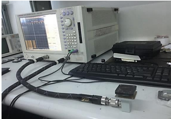
Gambar 3.30 Vector Network Analyzer (VNA) (Nuraini, 2015)
