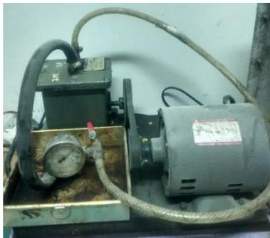
**Gambar 3.14** Pompa Vakum
