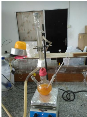
Gambar 4.7 Rangkaian Refluks Sintesis Biodiesel
