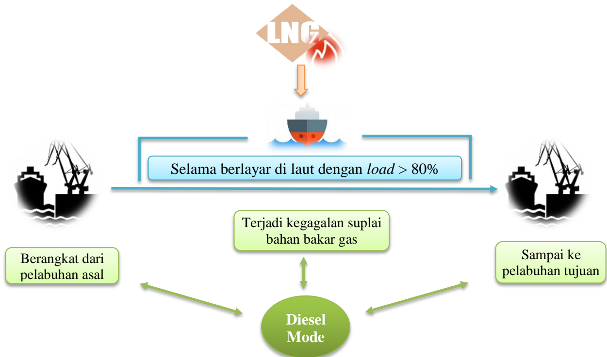
Gambar IV. 7 Skenario Penggerak Dual Fuel Self-Propelled Barge
