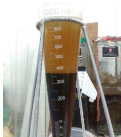
Gambar 4.1 Settleability Solid Test
