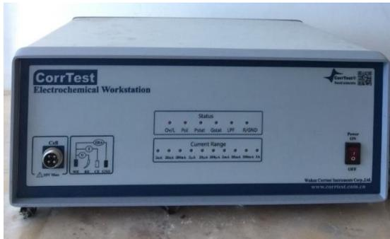
**Gambar 3.5** Alat Uji *Cyclic Voltammetry*
