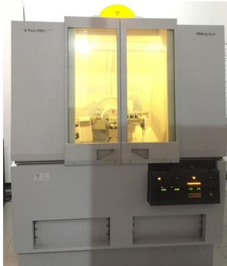
**Gambar 3.7** Instrumen XRD PANalytical
