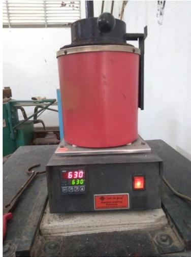
**Gambar 3.6** *Electric Melting Furnace*
