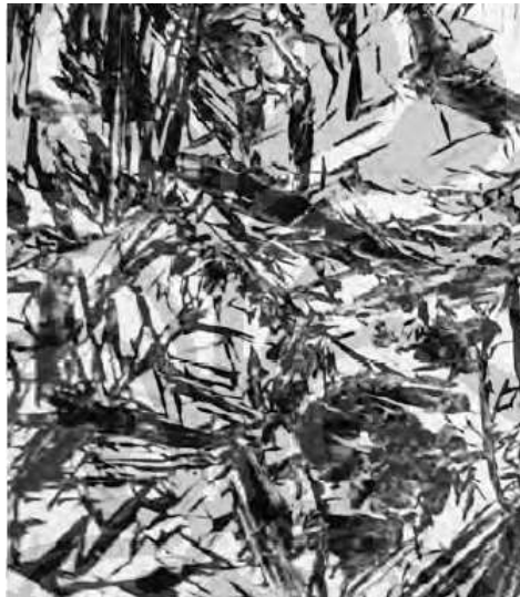
Gambar 2.9 Struktur Mikro Lath Martensit Hasil Quench. (Calister, 2007)
